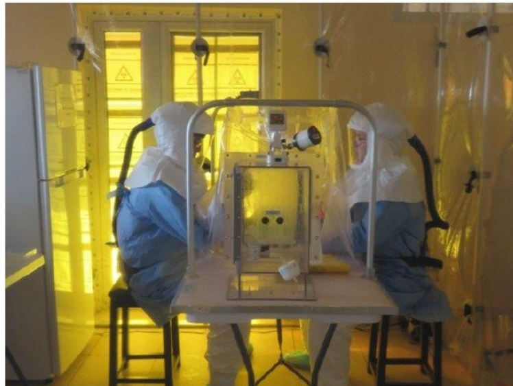
Figure 6: Professor Janusz Paweska and Dr. Petrus Jansen van Vuren performing inactivation of blood specimens submitted from suspected EVD patients in Freetown, Sierra Leone.
